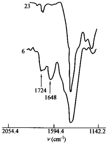
Fig. 1 IR spectra of Sample 6, 23 (crosslinked CPE) (CPE reacted with CH 3 COOK)
